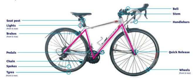
Follow the frame of the bike from the rear wheel up to the saddle, down to the pedals, up to the handlebars and down to the front wheel. This is your **M-check**.
